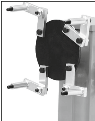
Install the 4 jaws on the black disk with the hexagon screws
